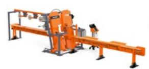
The TVS (Twin Vertical Saw) uses thin-kerf blades to efficiently remove the two vertical sides of logs up to 400mm in diameter. The TVS is cost-effective, versatile, designed for high performance, and built strong for years of reliable service. The TVS works equally well as a stand-alone unit or integrated with an existing sawmill line.
